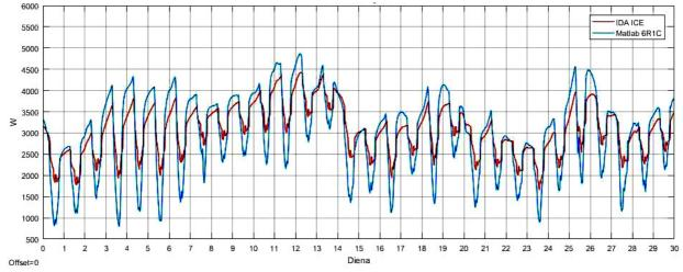
Fig. 3. Heating power variation of both models for same modelling period
