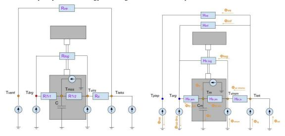
Fig. 1. Lumped 5R1C (left) and 6R1C (right) building thermal model
